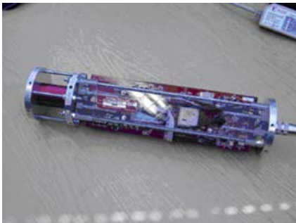
An example probe with detector (25mm x 40 mm), integrated digitizer and power supply.
